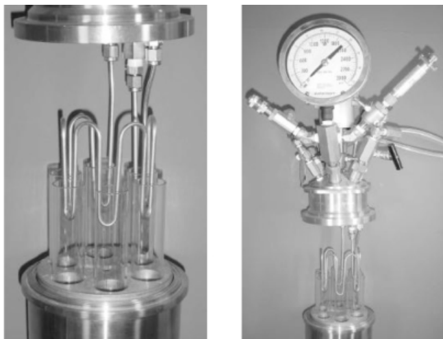
Figure 2. Six-fold parallel autoclave with aluminum insert and glass reaction tubes.
